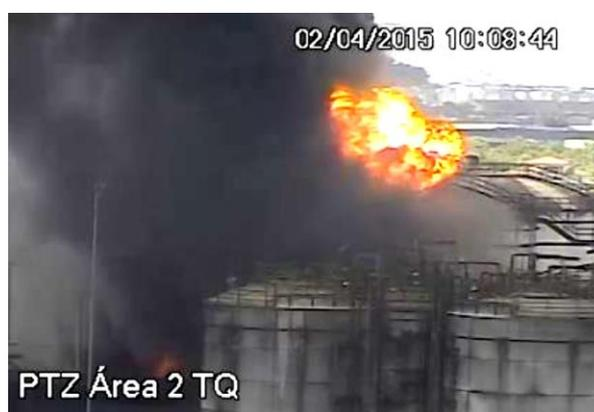
**Figura 12 – E) 10:08:44:** Fenômenos de UVCE (Unconfined Vapor Cloud Explosion).
